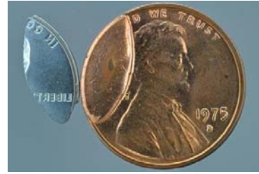
1975-D Cent with cud on the left where the piece of die shown broke away. //www.ngccoin.com. Photo courtesy of Dave Camire of NCS and Andrew Steiner of Harlan J. Berk, ...
