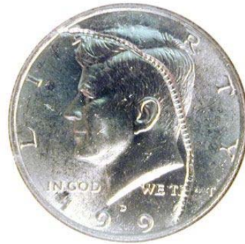
Example of strike through error 199X-D Kennedy Half-Dollar. www.pinterest.com
