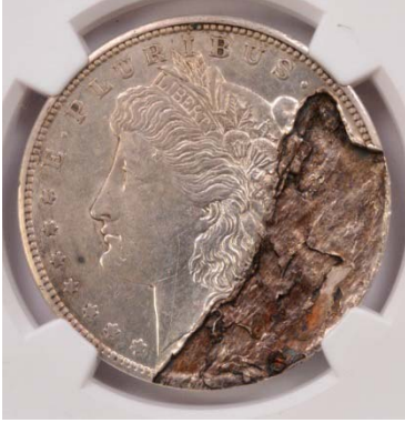
Lamination error on 1921-S Morgan Dollar - https://sullivannumismatics.com
