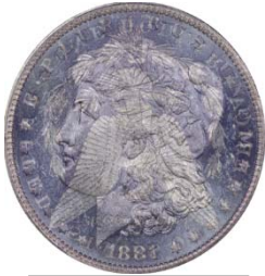
Clashed Die error on 1881-O Morgan Dollar. http://www.1881o.com/clashing.html
