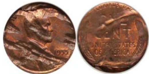
Sample of defective planchet - http://coinauctionshelp.com
