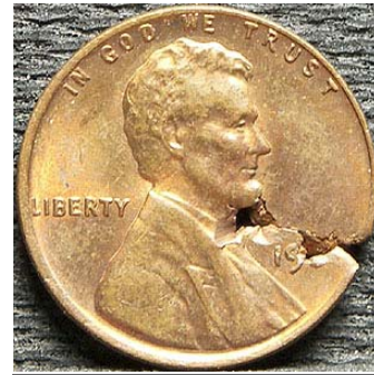
Sample of defective planchet http://www.lincolncentresource.com
