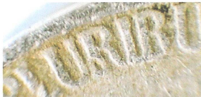
Two magnified views of the die defect on the reverse of the Henning coins. Note the bubble near the bottom of the "R" in Pluribus. Apparently, the same reverse die was used on all of Henning's coins, so this defect should be present on all 6 dates: 1939, 1944, 1946, 1947, 1953 and the mystery 6th date.
