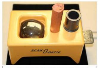
Close up of the Scan-O-Matic. This device came with different size insert tubs (black tube on right) to fit the various denominations of coin.
